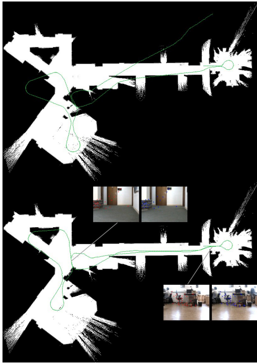
Fig. 9. Example of a topo-metric map included in a laser map for reference (sequence Lab). (a) raw odometry, (b) trajectory corrected using our algorithm. The length of the trajectory was about 96 meters.
