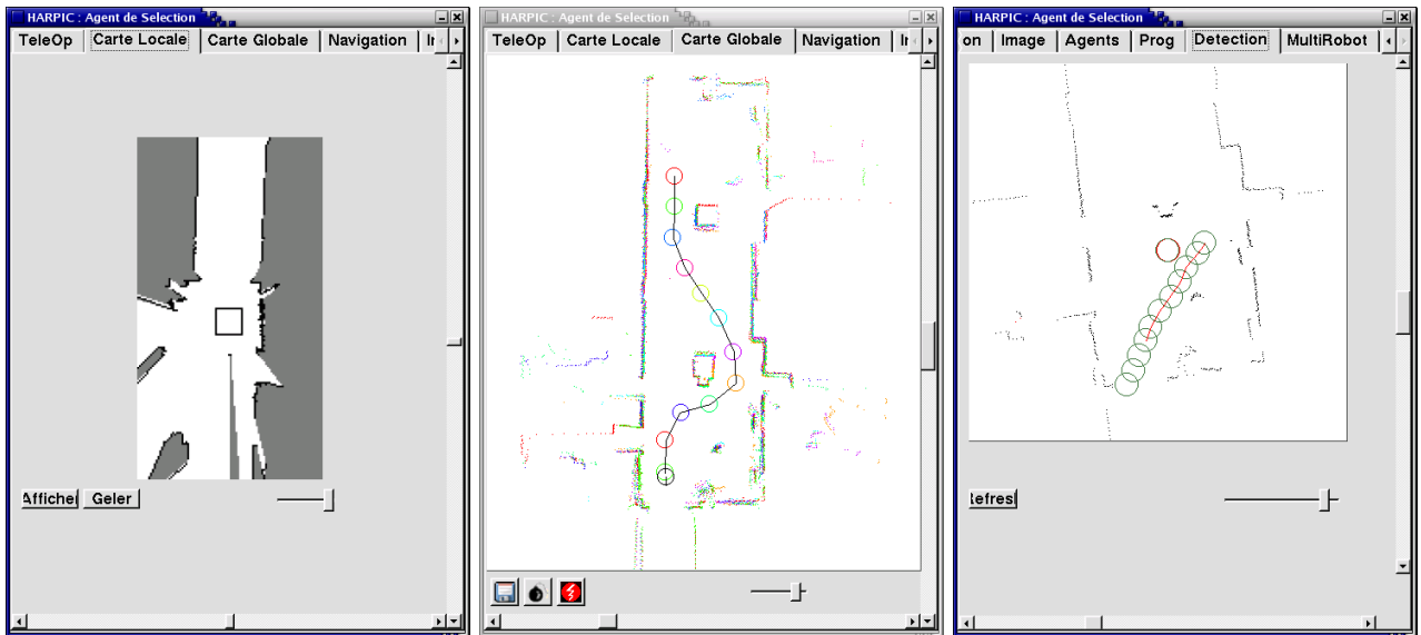
Figure 5. Interface for local map (left), global map (center) and moving object detection (right).
