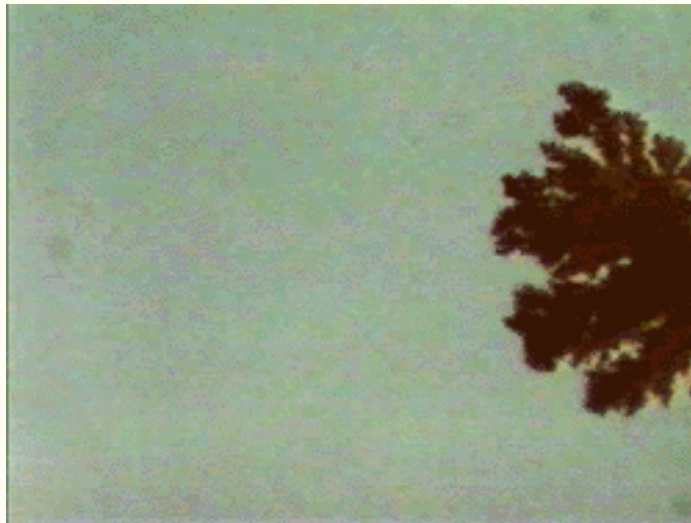
Copper sulfate electrochemical deposition viewed through a microscope
